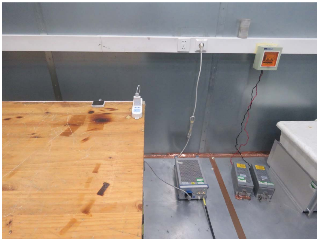
Picture 2 Conducted Emission Test Setup
