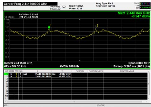
BT DH5 CH39, Carrier frequency (MHz): 2441
