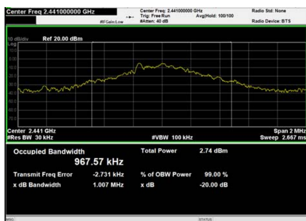
BT DH5 CH39, Carrier frequency (MHz): 2441
