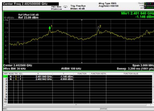
BT DH5 CH78, Carrier frequency (MHz): 2480
