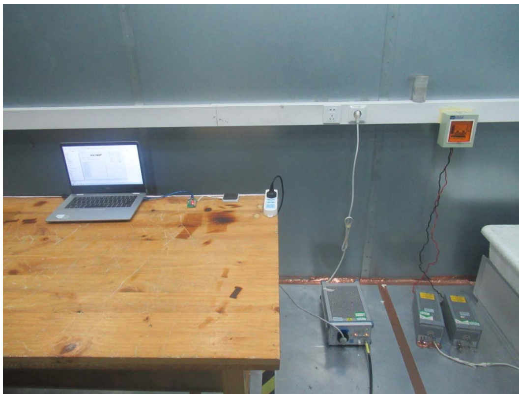
Picture 2: Conducted Emissions Test Setup
