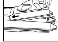
Put cover of main cabin onto its proper place and press the edge to fix it well.
