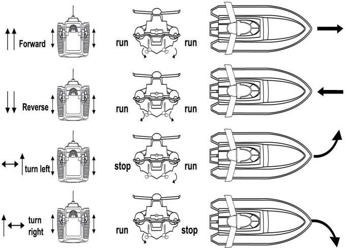
Pull up throttle stick, two propeller run and the boat drives forward. Then pull down throttle stick, the propellers stop working and the boat slows down. Pull direction control stick to the left, propeller on the boat's left side stops working but propeller on the right side runs, the boat turns left; then pull direction control stick to the right, propeller on the boat's right side stops working but propeller on the left side runs, the boat turns right instead.
