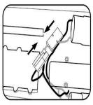
③ Plug battery to the socket of the receiver.
