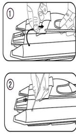
Put antenna cord through PVC tube and then insert the PVC tube into the hole on the hull.
