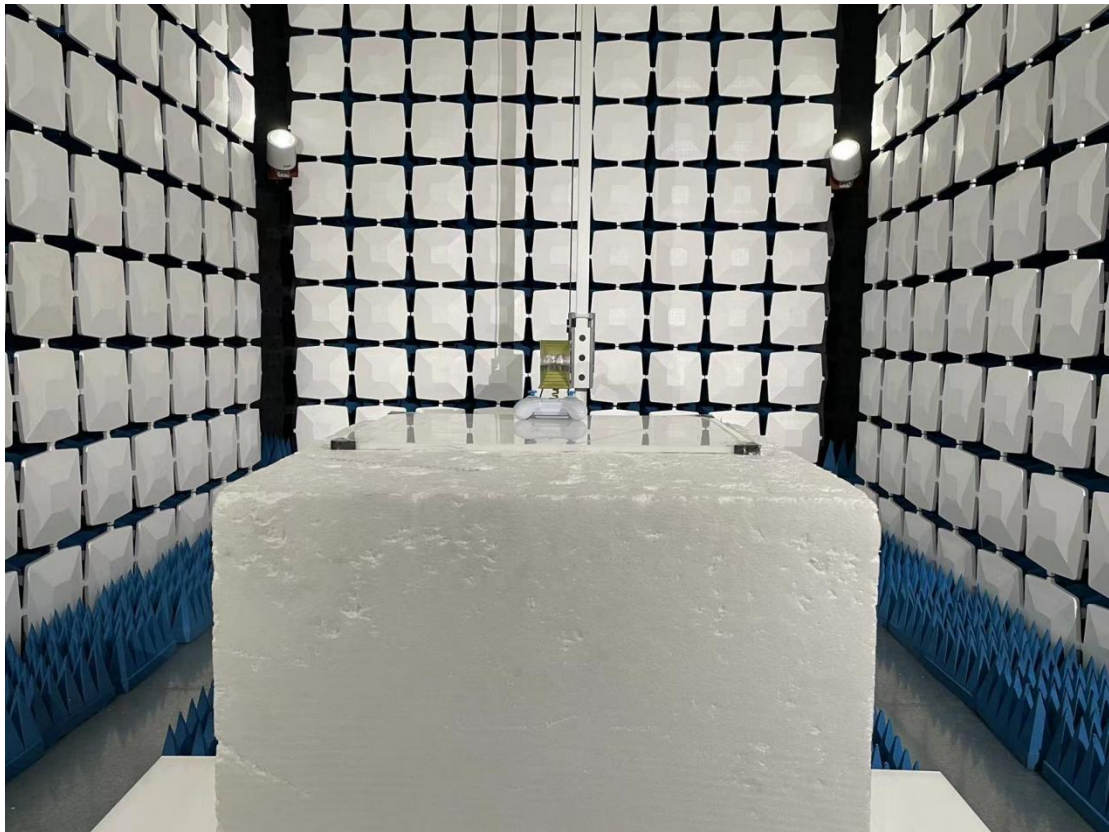
Above 1GHz for radiated emission test setup
