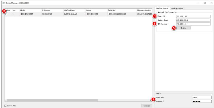
**NOTE:** Before entering the IP address, please go to WIN+R->CMD->ipconfig/all->Scroll down to Ethernet Adapter and check the IP address like 192.168.X.97 of your PC, then it'll be okay to enter the IP like 192.168.X.96 for the encoder and click "Modify", generally it's on the same network segment and okay to access the encoder.
