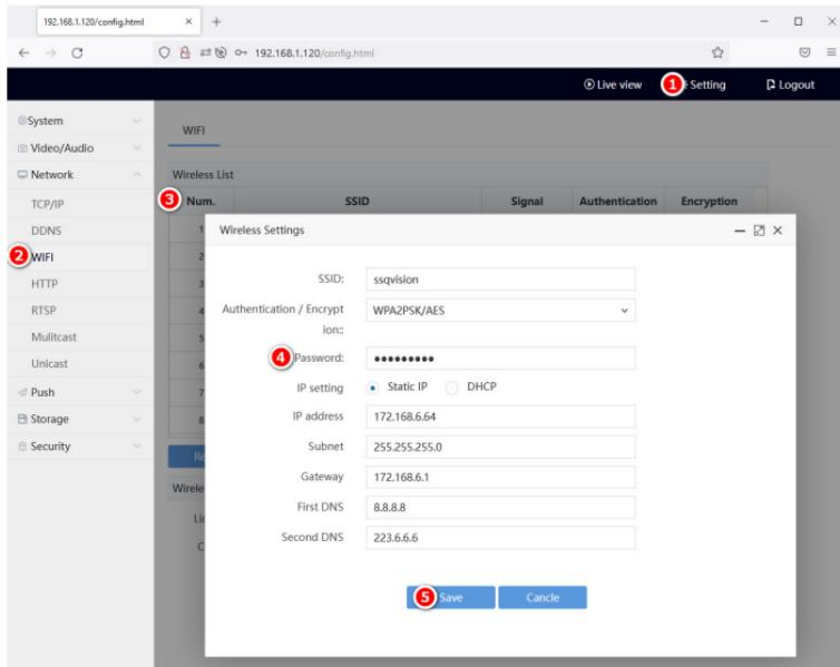
**NOTE:** It's necessary to plug out the ethernet cable and power off the encoder to reboot it to make WiFi valid.
