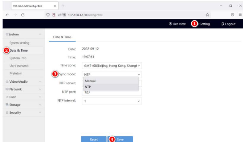
**NOTE:** It's necessary to set date and time no matter whether it's synchronized with the PC time or manually set, or else the below recording won't be valid and searched.
