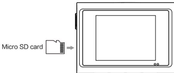
Please make sure the camera is turned off first. Then align the gold-plated contacts facing towards the back of the camera (Screen Side).
