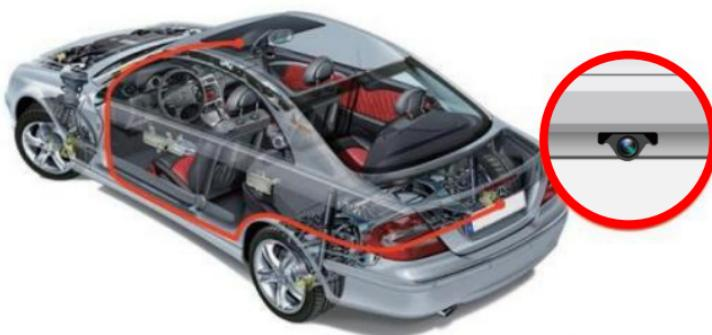
5. Plug the supplied car charger into your vehicle's accessory port and the other end into the micro USB port. Route the cable alongside the interior trim for better looking.
