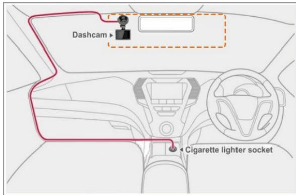
2. Clean the spot on your windshield where you want to mount the camera and confirm the placement. We recommend installing the camera near the rear view mirror of the driver's opposite side.
