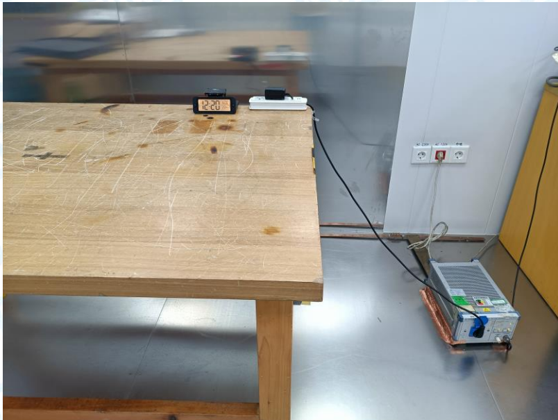
Photo of Setup for Conducted Emission
