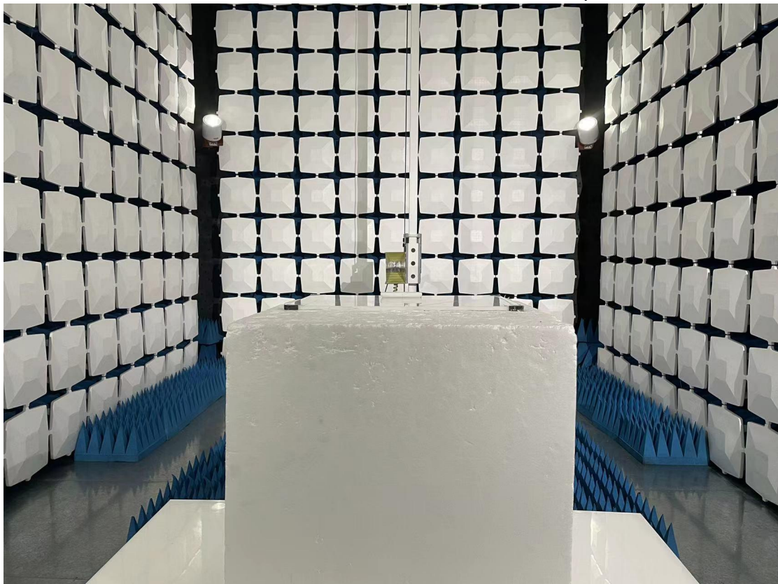
Above 1GHz for radiated emission test setup
