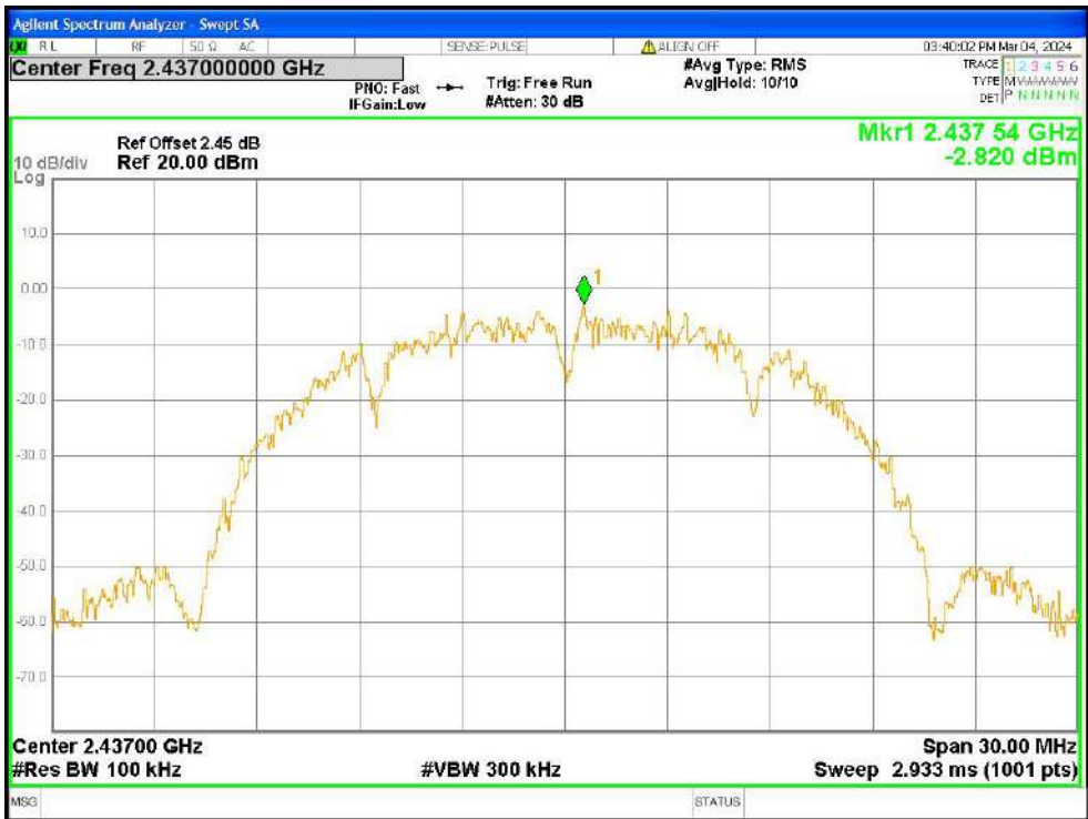
Tx. Spurious NVNT b 2437MHz Ant1 Ref
