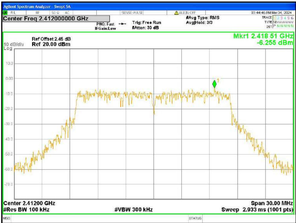
Tx. Spurious NVNT g 2412MHz Ant1 Ref
