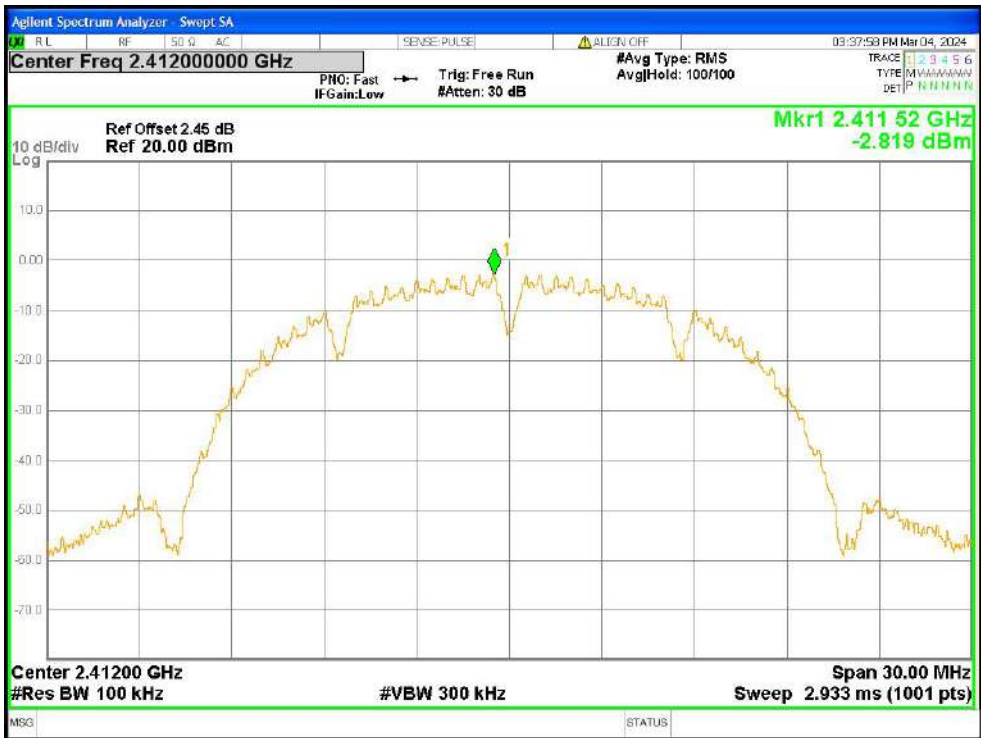
Tx. Spurious NVNT b 2412MHz Ant1 Ref
