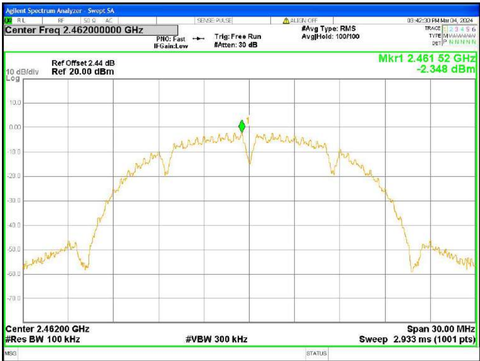
Tx. Spurious NVNT b 2462MHz Ant1 Ref
