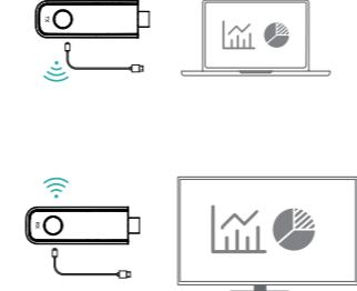
1. Connect the HD port of the receiver to the video input port of the display device such as the monitor or TV.
