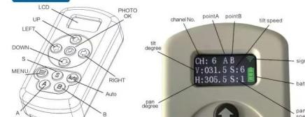
First power on pan tilt, then power on the remote. The remote signal turns green if the pan tilt channel No. is the same as the remote channel No. When the signal is green, the remote can be used. If the pan tilt channel No. is inconsistent with remote channel No. The red character "SELECT CH" will blink on LCD. Simultaneously the channel No. also blinks. Press UP or DOWN key to change the remote channel, when it is the same channel as pan tilt press OK to confirm.
