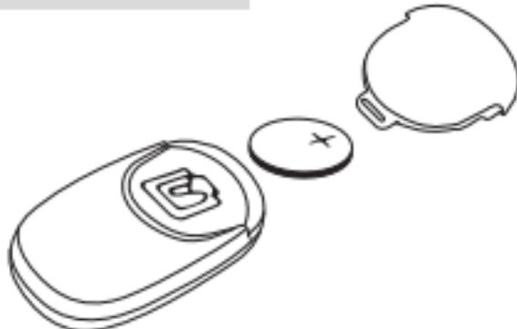
Positive pole upwards to install the battery.
