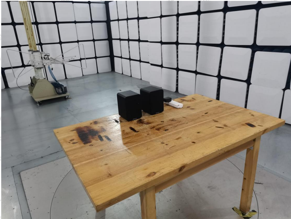
Photo of Radiation Emission Test
