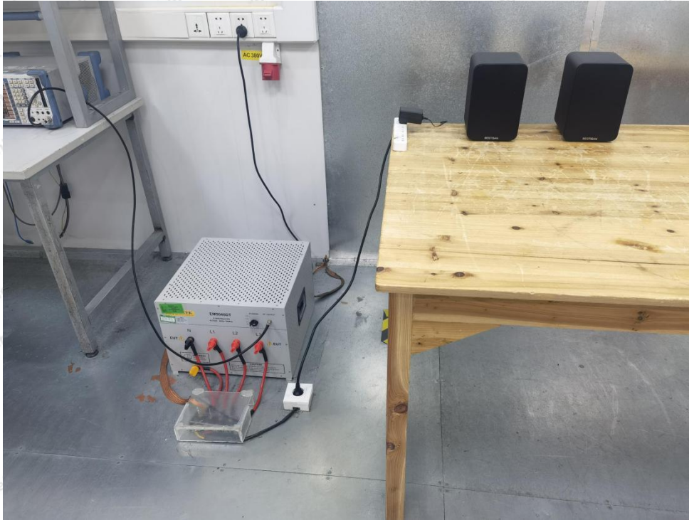
Photo of Conducted Emission Measurement
