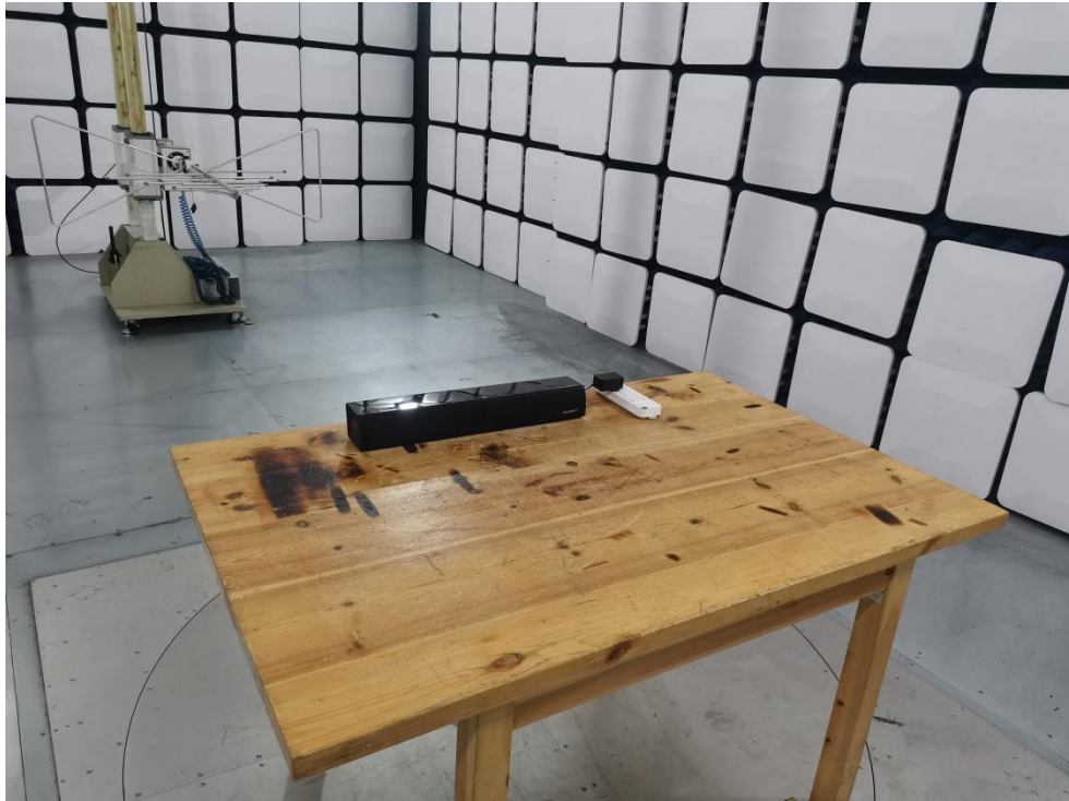
Photo of Radiation Emission Test
