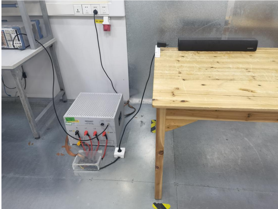
Photo of Conducted Emission Measurement
