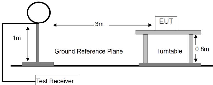
For Radiated Emission 30-1000MHz
