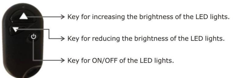
When pressing **▲** and **▼** simultaneously, the LED lights will flash.
