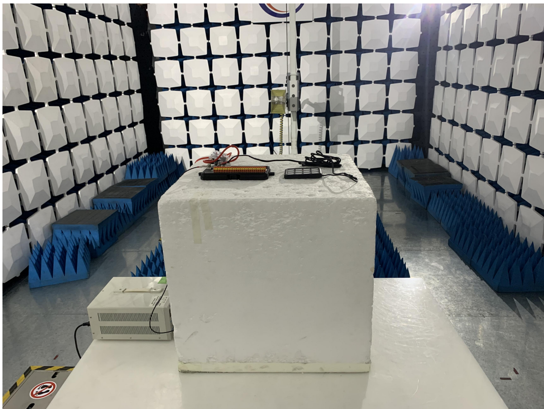
Above 1GHz for radiated emission test setup
