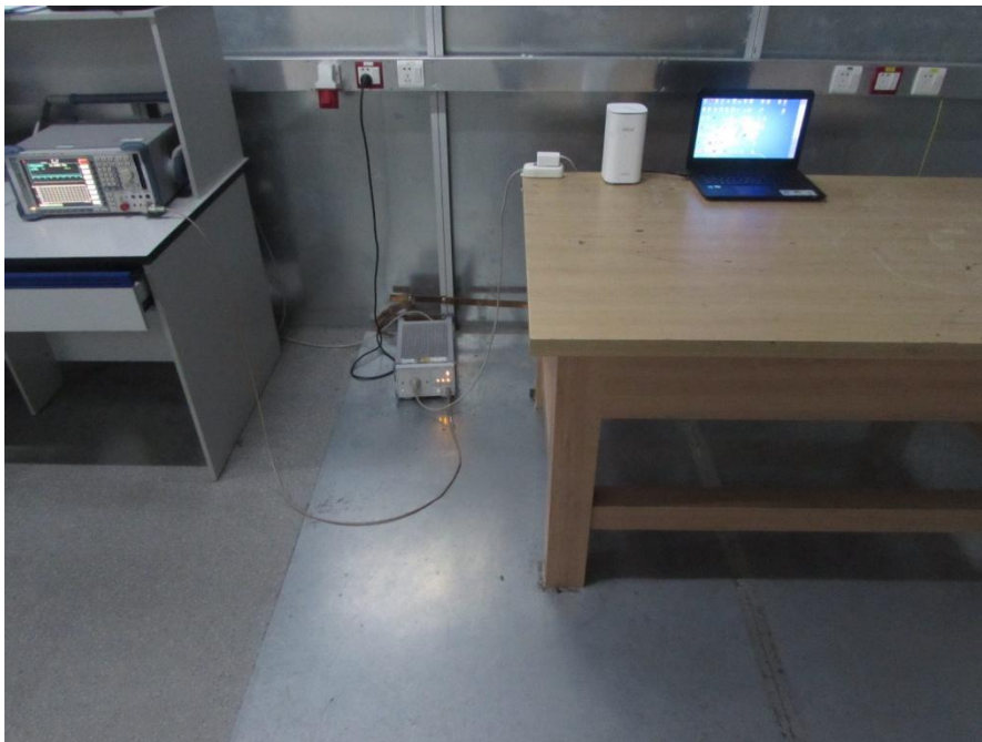
CONDUCTED EMISSION TEST
