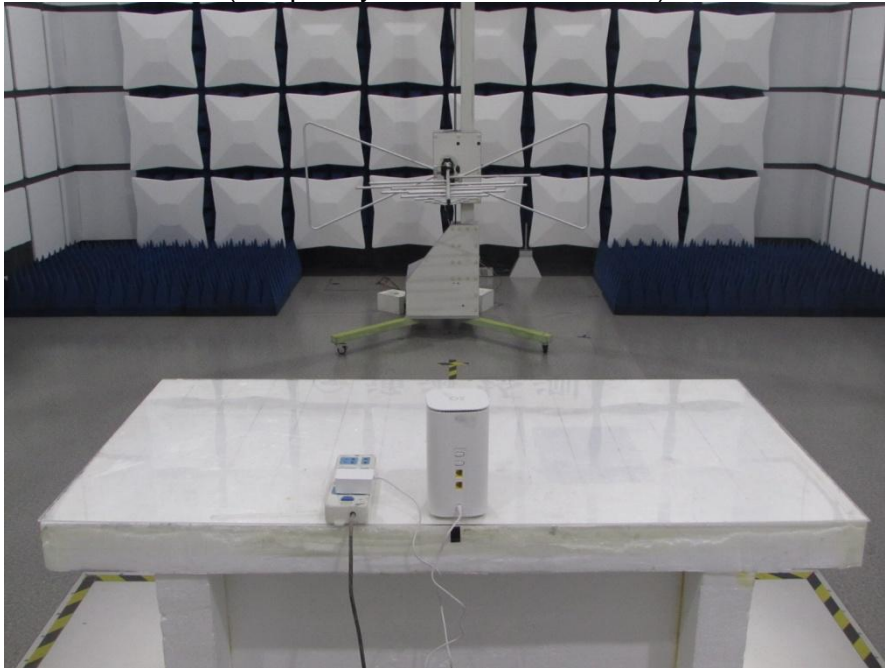
RADIATED EMISSION TEST (Frequency from 30MHz to 1GHz)
