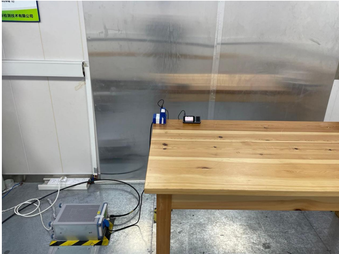
Conducted emission test setup
