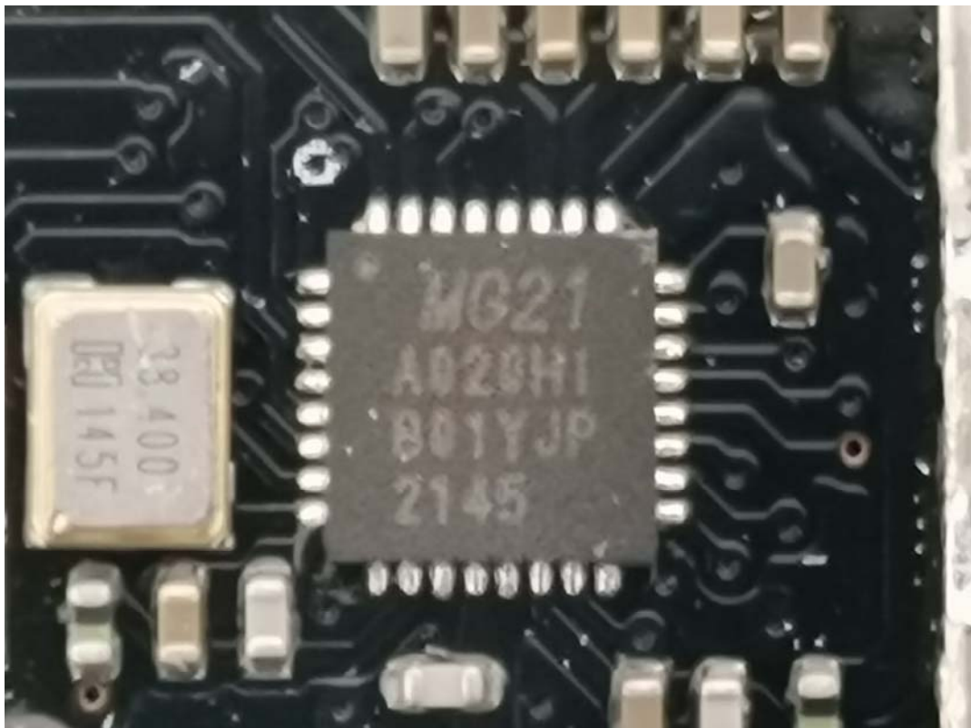
ZigBee RF Chip
