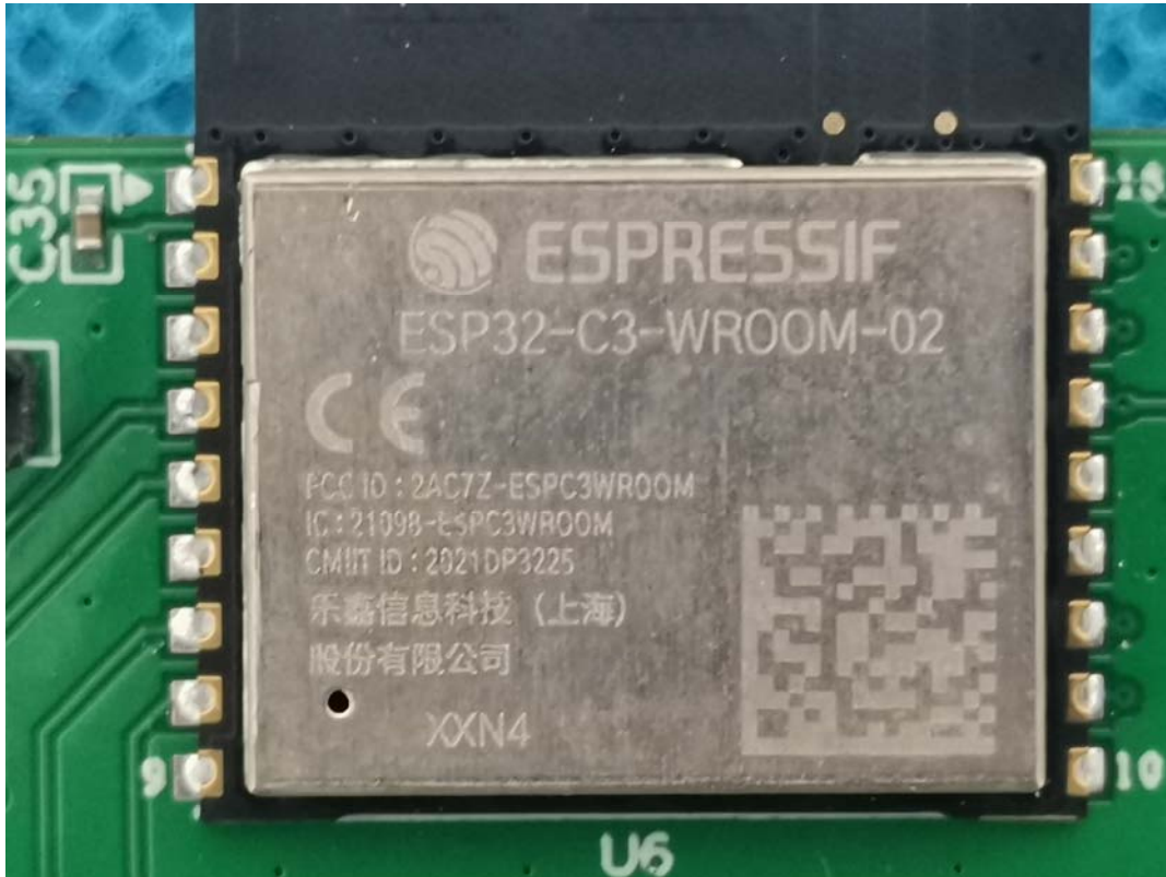
BT&Wi-Fi Module unshielded View
