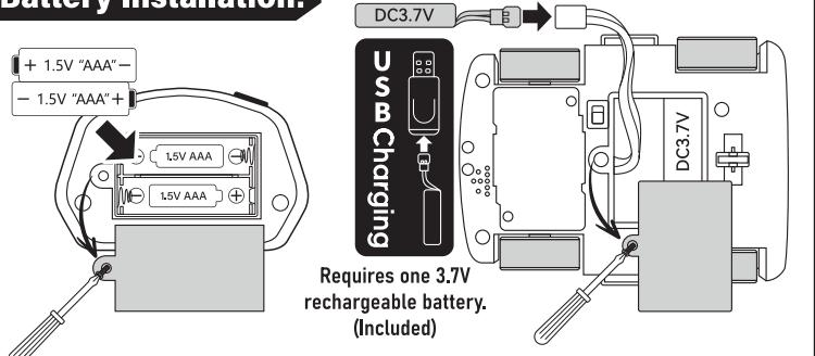
1. Insert 2 x 1.5V "AAA" batteries into the battery compartment of the remote controller with correct polarity.
