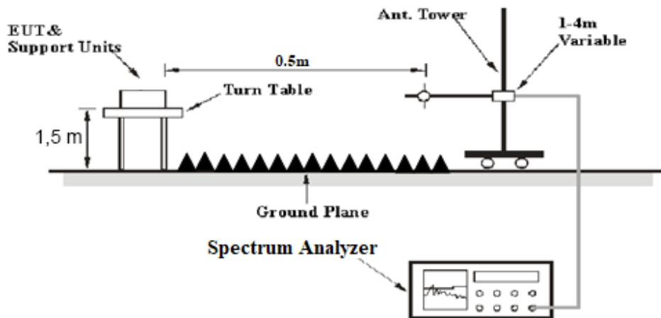
The antenna is scanned around the entire perimeter surface of the EUT, in both horizontal and vertical polarizations, at the distance of 2 m from 1 GHz to 18 GHz, and 0.5 m from 18 GHz to 40 GHz.
