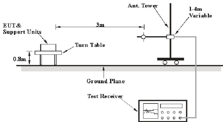
The radiated emission below 960MHz tests were performed in the 3 meters chamber test site A, using the setup accordance with the ANSI C63.10-2013. The specification used was the FCC 15.209 limits.
