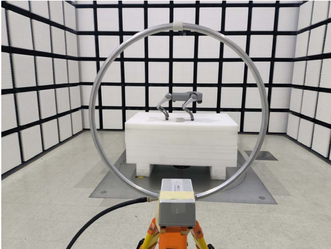
Radiated Emission 9kHz-30MHz View-Perpendicular
