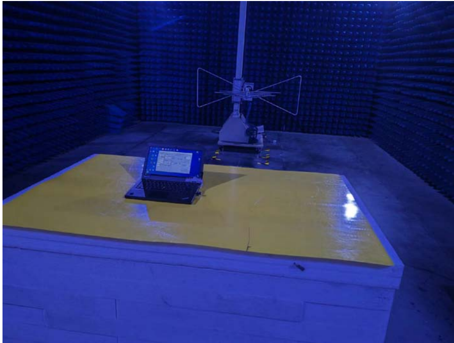
Photo of Radiated Emission Measurement Below 1GHz
