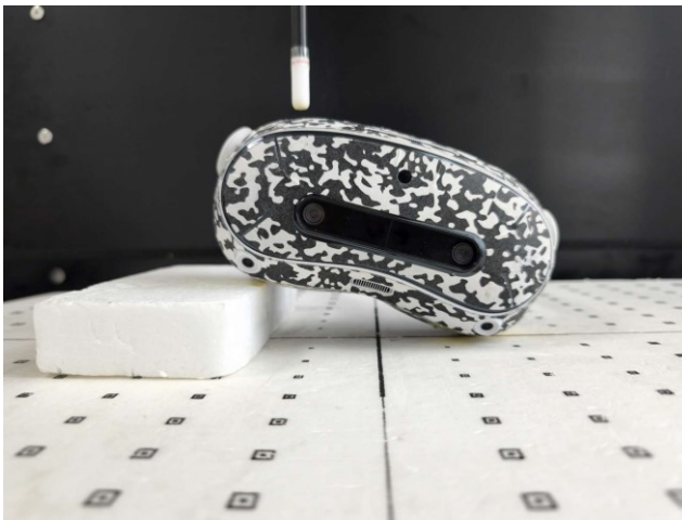
Top Side position2, Test Separation 8.59 mm
