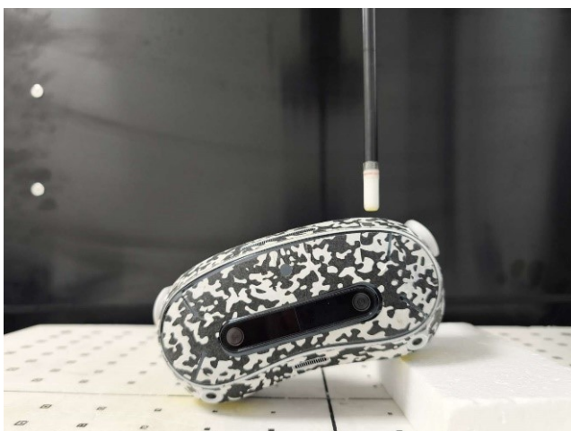
Top Side position1, Test Separation 2 mm
