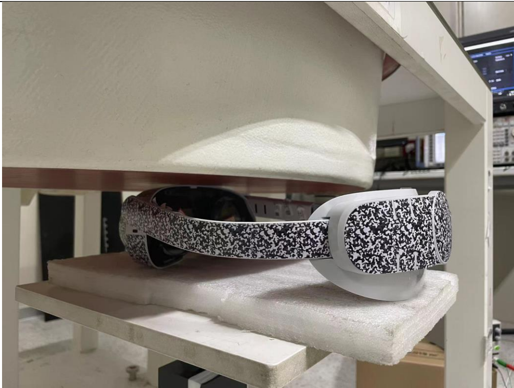
SAR Set-up Photo -Side 1
