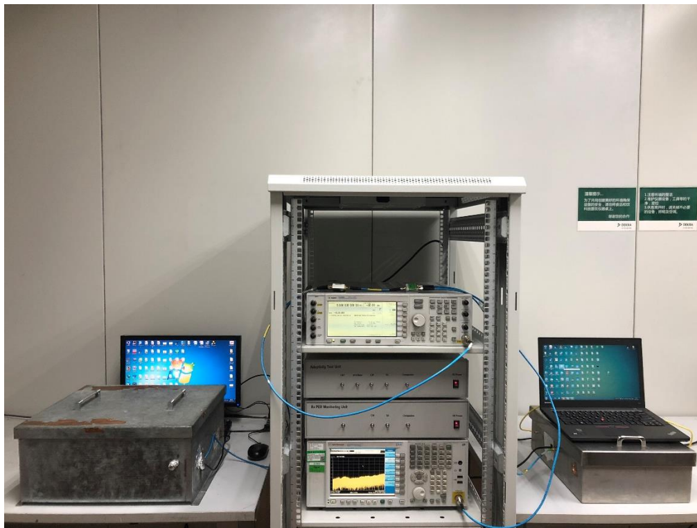
DFS Set-up Photo: Slave and Spectrum Analyzer
