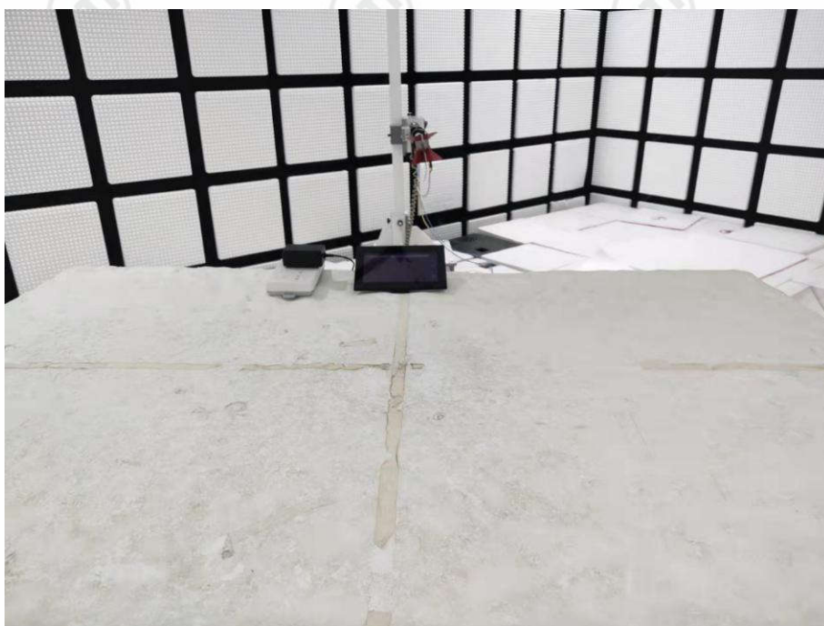
Radiated spurious emission Test Setup-2(Above 1GHz)
