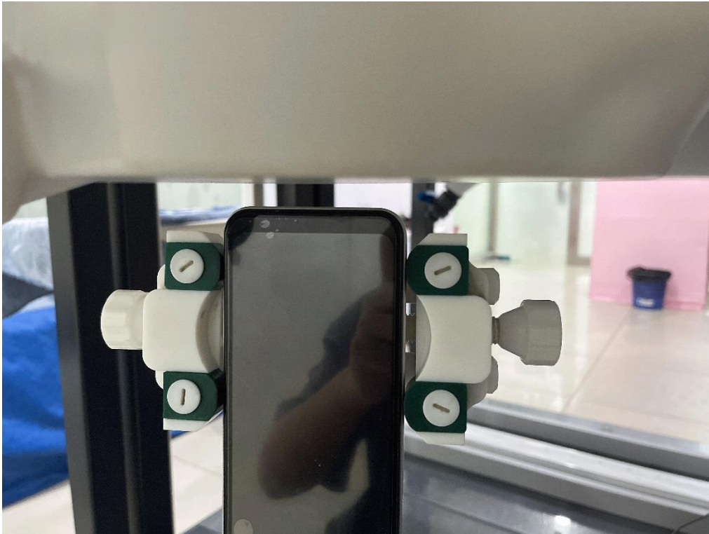
Body Bottom side(separation distance is 10mm)
