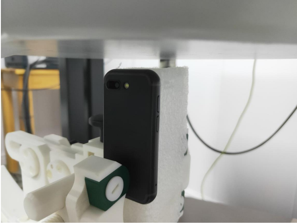
10mm body-worn Top Side Setup Photo (hotspot)
