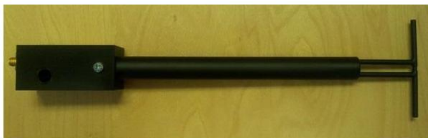
Figure 1 – MVG COMOSAR Validation Dipole
