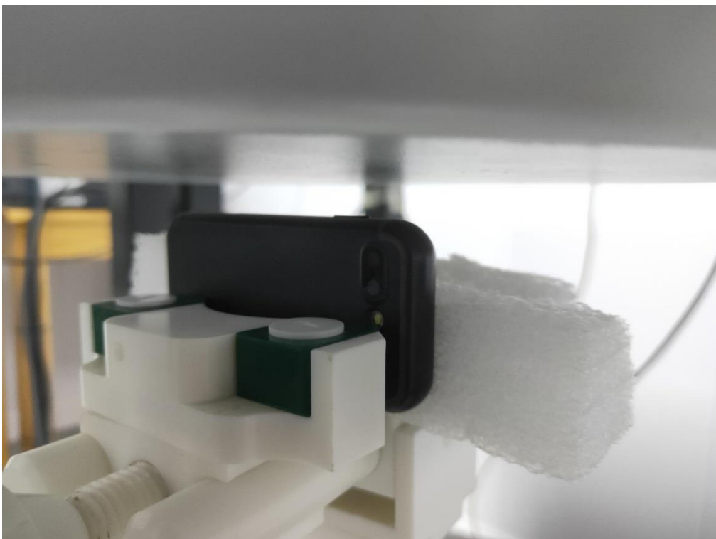
10mm body-worn Right Side Setup Photo (hotspot)
