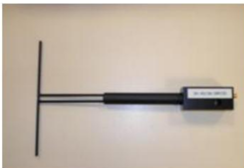
Figure 1 – Satimo COMOSAR Validation Dipole
