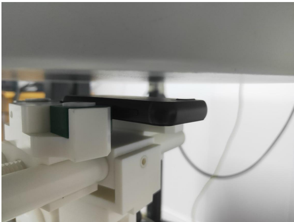
10mm body-worn Back Side Setup Photo(hotspot)
