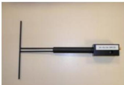
Figure 1 – Satimo COMOSAR Validation Dipole
