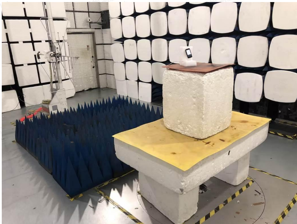
Radiated Emissions Measurement (Below 1GHz)
