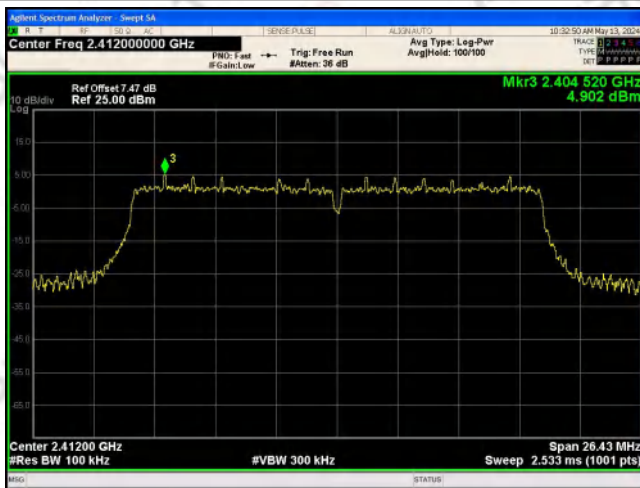
In-Band Reference Level IEEE 802.11n_Channel 1_20MHz_Antenna 0
