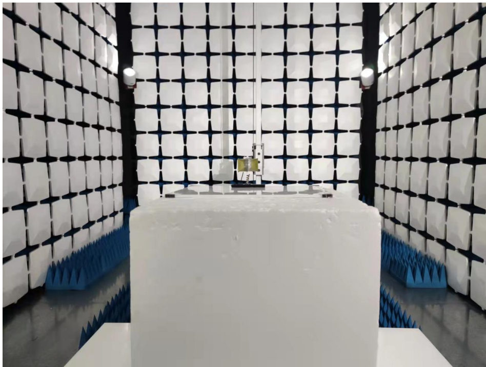
Above 1GHz for radiated emission test setup
