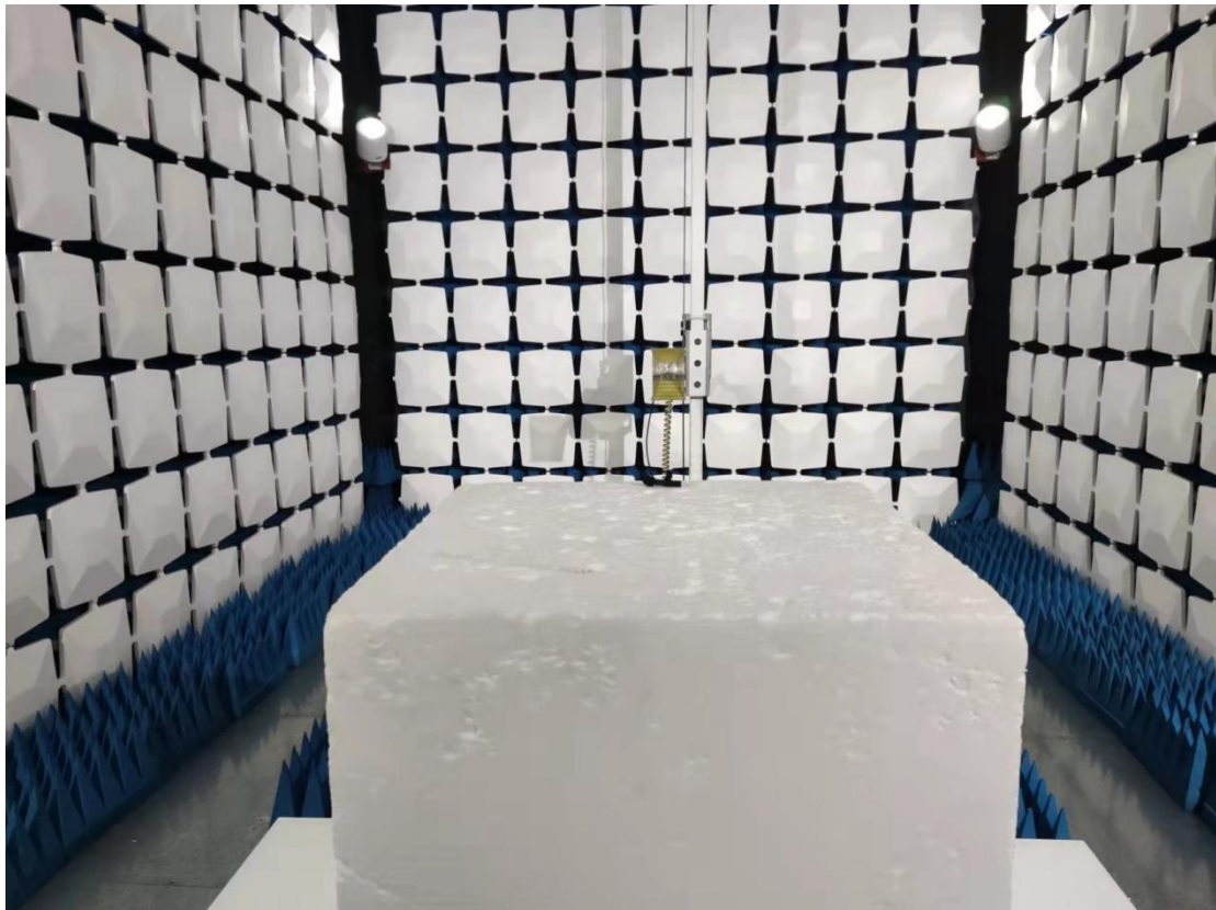
Above 1GHz for radiated emission test setup
