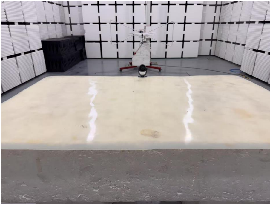
Set-up for Radiated Spurious Emission, Above 1GHz
