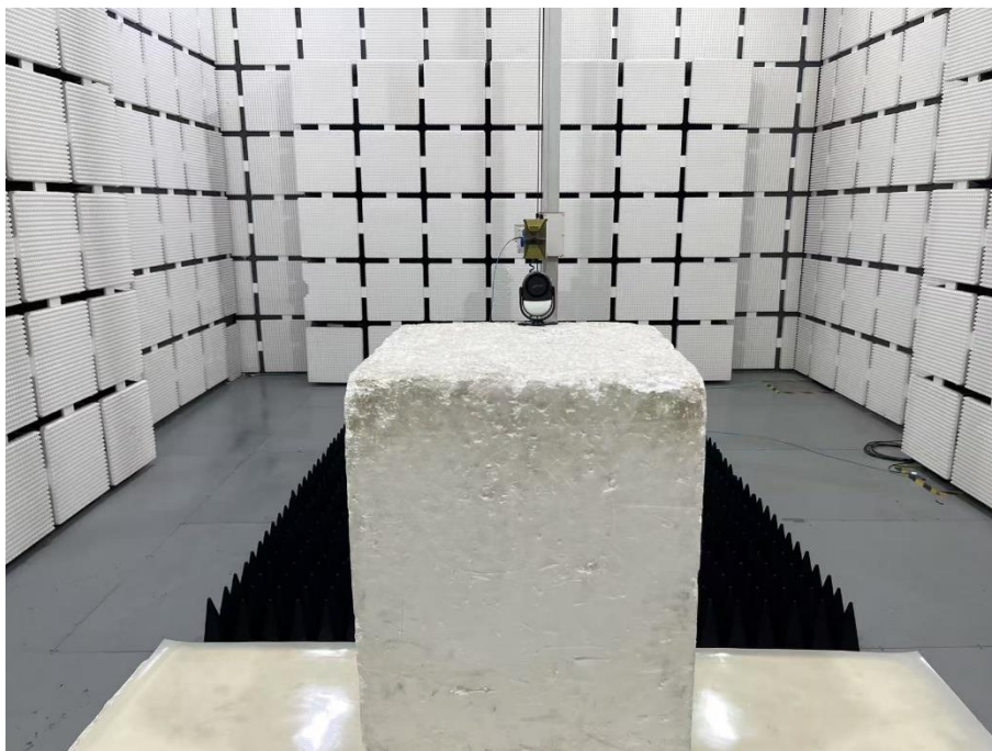
Set-up for Radiated Spurious Emission, Above 1GHz
