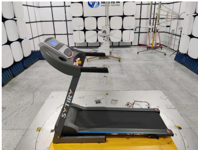
Radiated Spurious Emissions From 30M-1GHz
