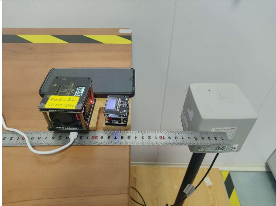
Test setup of C side
