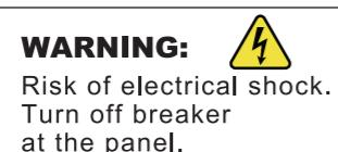
Switch off the main electrical supply from the fuse box/circuit breaker before installing the unit or doing any maintenance.
