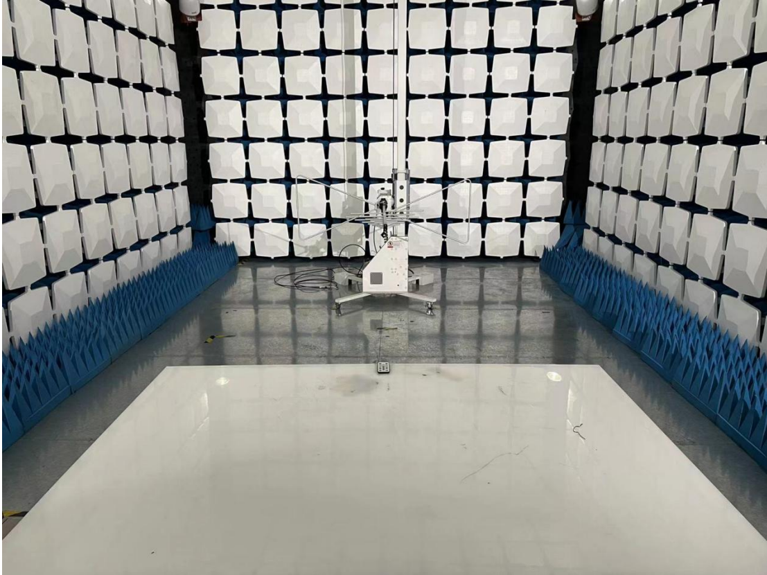
Above 1GHz for radiated emission test setup
