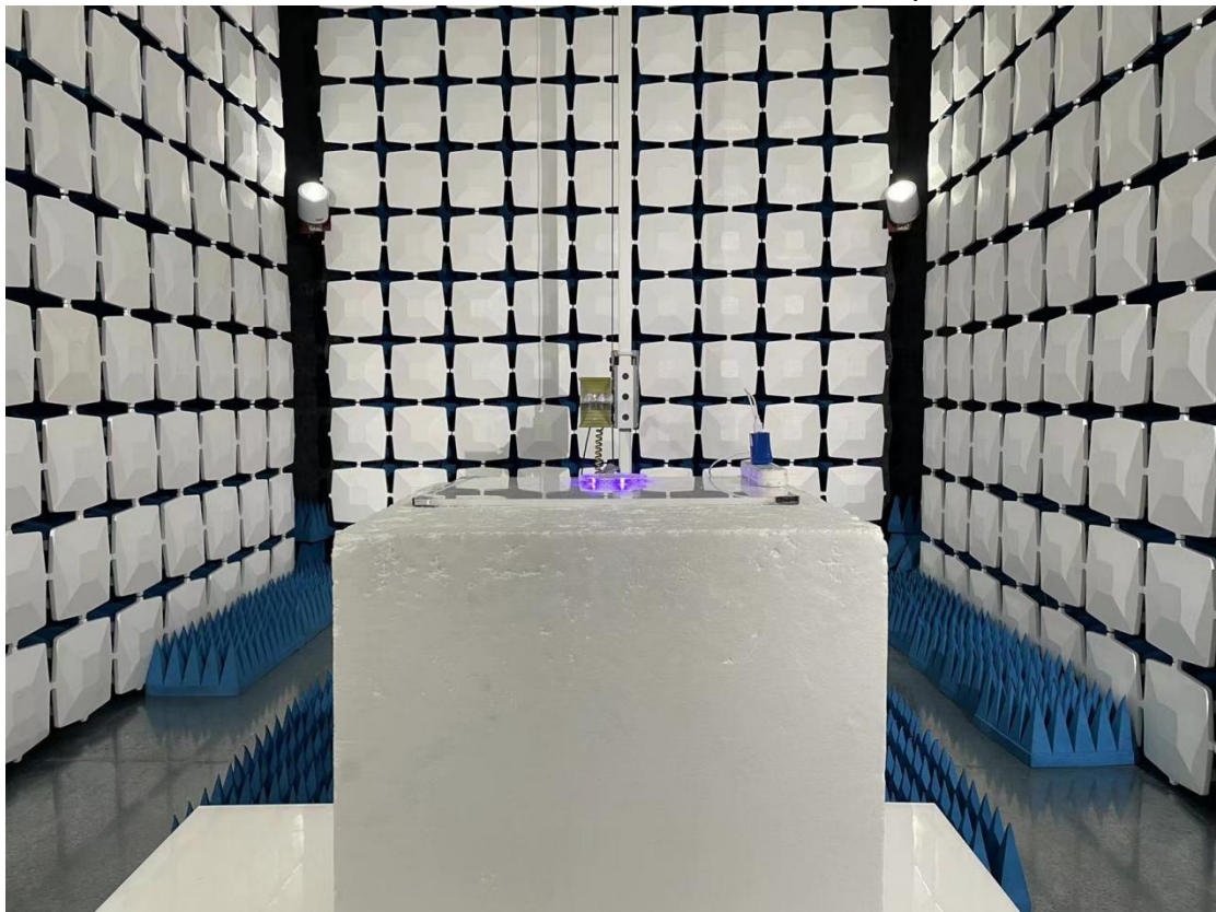
Above 1GHz for radiated emission test setup
