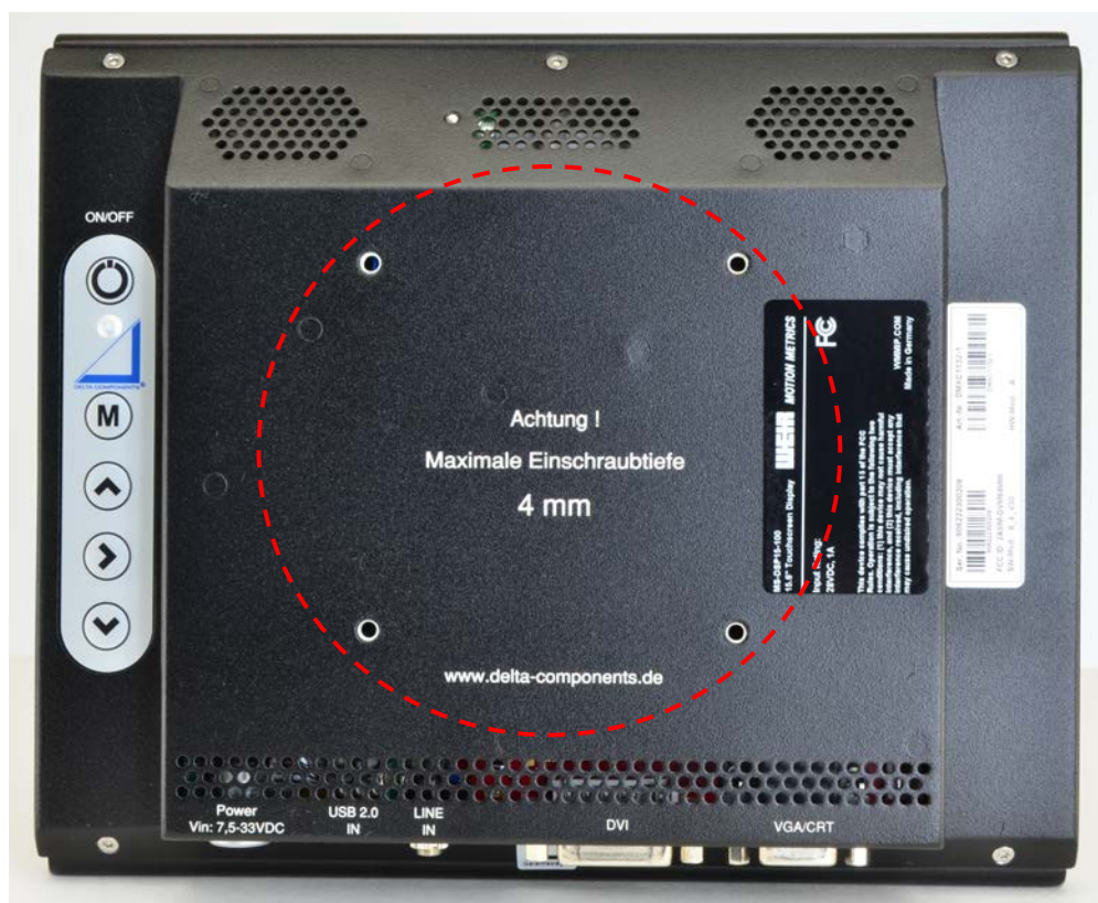
Figure 12: VESA Mounting on the rear side
