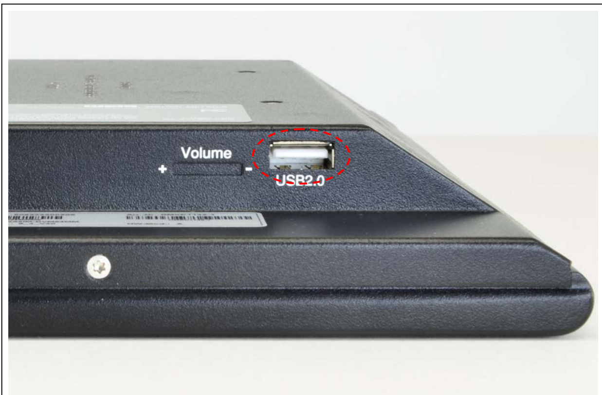
Figure 11: USB Type A Interface on the left side of the monitor
