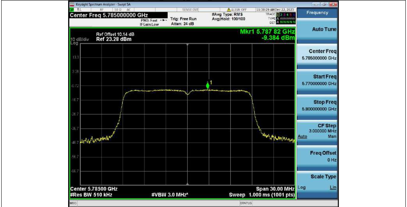
Power Spectral Density NVNT ANT1 802_11n(HT20)_5785
