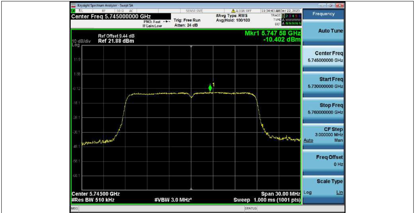
Power Spectral Density NVNT ANT1 802_11n(HT20)_5785
