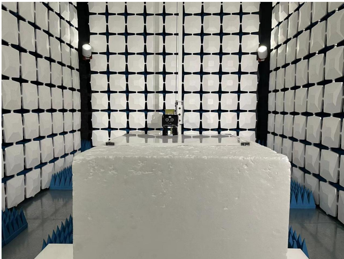
Above 1GHz for radiated emission test setup
