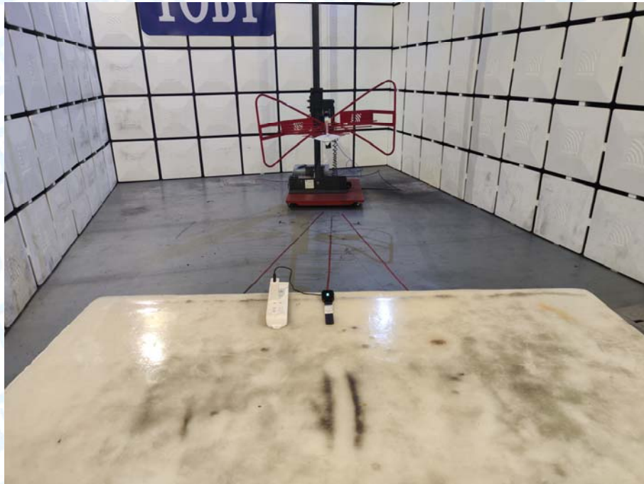
Photo of Setup for Conducted Emission
