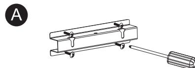
A: First, use the screws in the accessory bag to fix the pegboard parallel to the pre-installed position of the equipment. It is recommended that the optimal height for installation is greater than the height of the pet.
