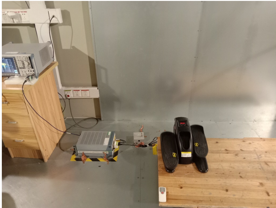
Photograph of test setup for Conducted Emission
