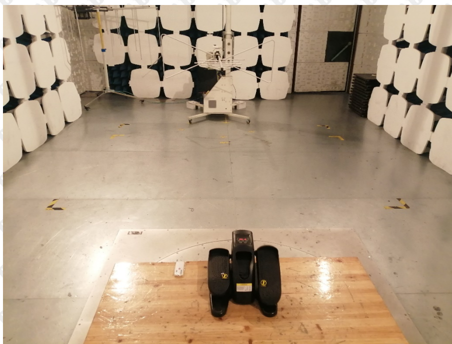
Photograph of test setup for Radiated Emission below 1 G
