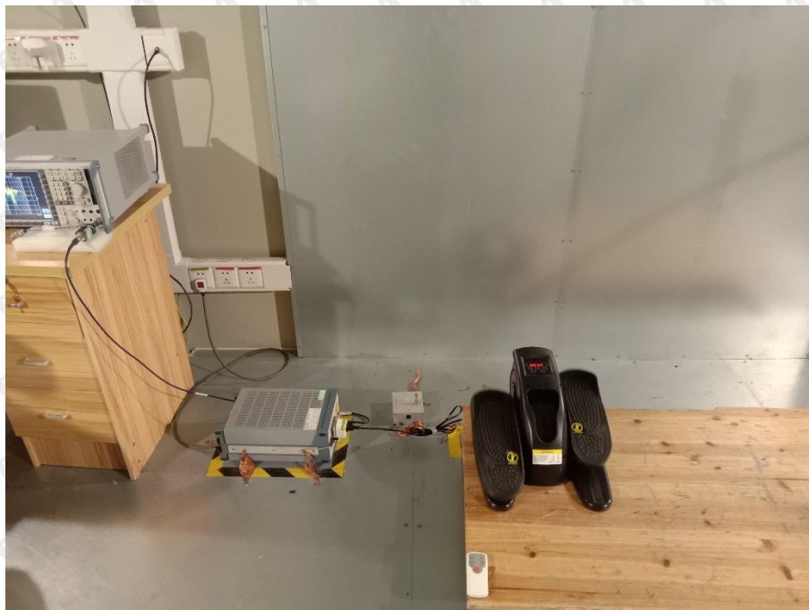
Photograph of test setup for Conducted Emission
