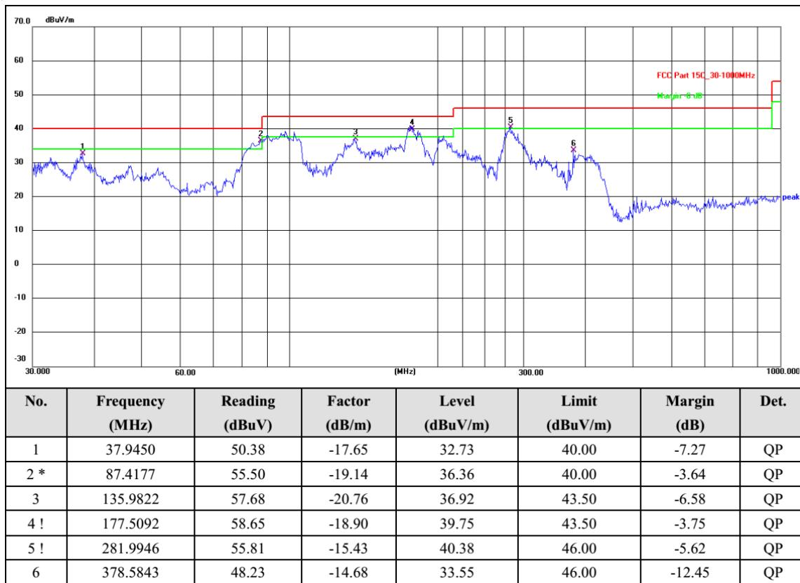
1). Emission level (dBuV/m) = 20 log Emission level (uV/m).
